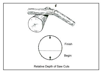
Figure 3. Crosscutting Logs/Limbs with Pressure on Bottom
